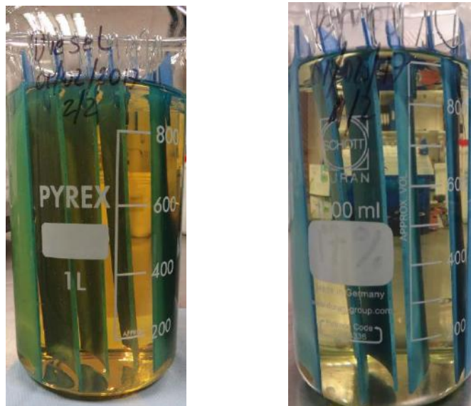
Figure 1 CCH5 in diesel (on the left) and petrol (on the right) - immediately after submersion
